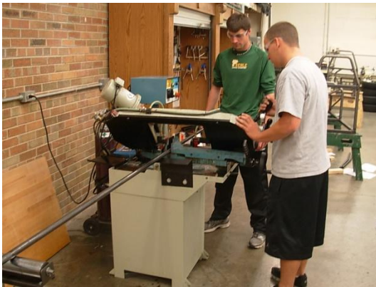
Devan and Matt cutting 1 ½" tubing for a support brace on the front of the chassis.
